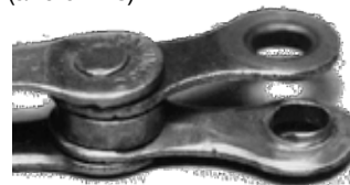
Chain with pin completely removed (avoid this)
